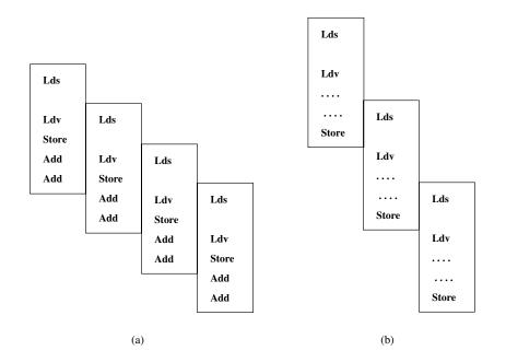
Figure 6: Software pipeline using lds/ldv
