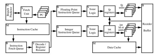
**Figure 1.** SMT processor hardware (diagram adapted from [25]). Each shared hardware resource is labeled with a letter signifying one of three resource classes: instruction slots (S), instruction buffers (B), and memories (M).
