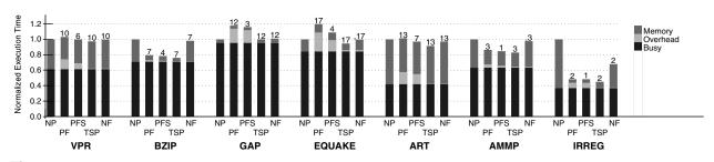
**Figure 8.** Normalized execution time for different prefetching schemes: no prefetching (NP), naive conventional software prefetching (PF), selective conventional software prefetching (PFS), Transparent Software Prefetching (TSP), and TSP without foreground thread flushing (NF). The label appearing above each bar reports the number of instrumented loops.
