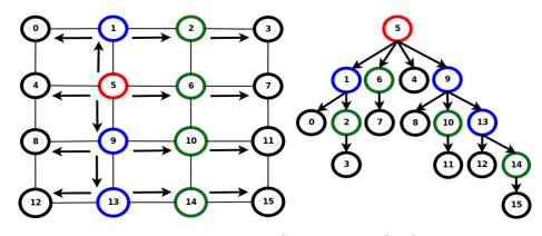
Figure 3.5: Broadcast Tree: Static Routes Configuration
