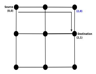
Figure 1.4: XY Dimension Order Routing
