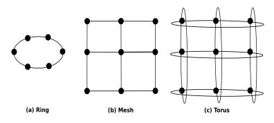
Figure 1.2: Common NoC Topologies
