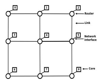
Figure 1.1: Network-on-Chip Architecture
