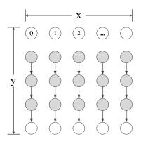
Figure 4.7: Communication Pattern of a 2D Stencil Code
