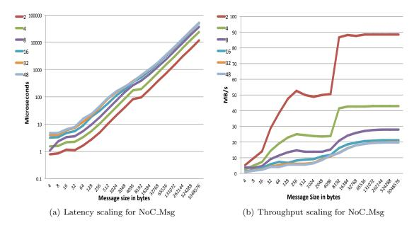
Figure 6.3: Scaling analysis for *bcast()* of NoC\_Msg
