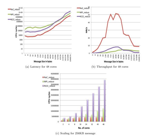
Figure 6.4: Performance analysis for reduce() of NoC\_Msg, RCKMPI and RCCE
