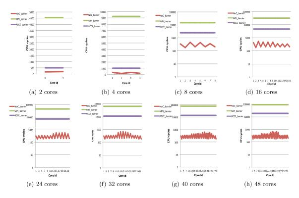
Figure 6.9: Scaling performance for *barrier()* of NoC\_Msg, RCKMPI and RCCE
