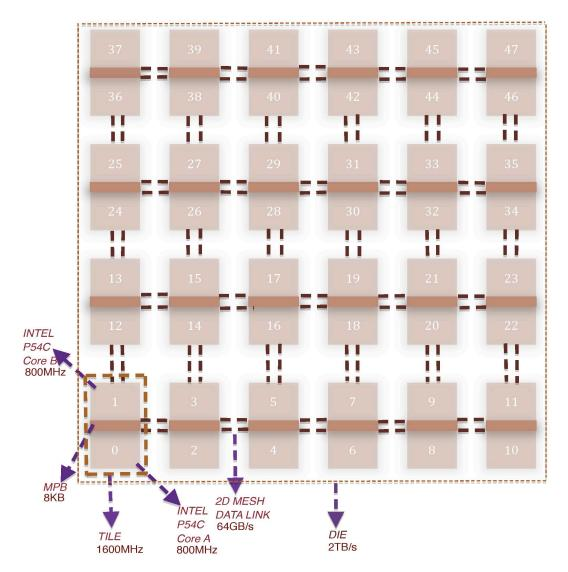
Figure 2.1: Intel SCC architecture schematic
