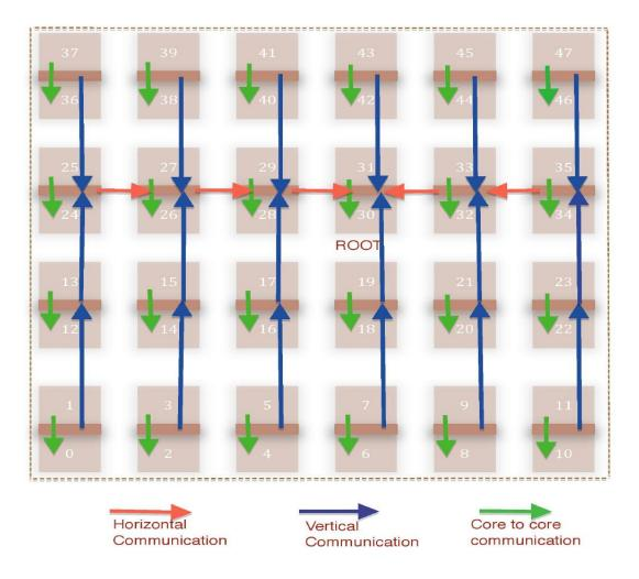
Figure 4.2: Communication pattern of Reduce on Intel SCC
