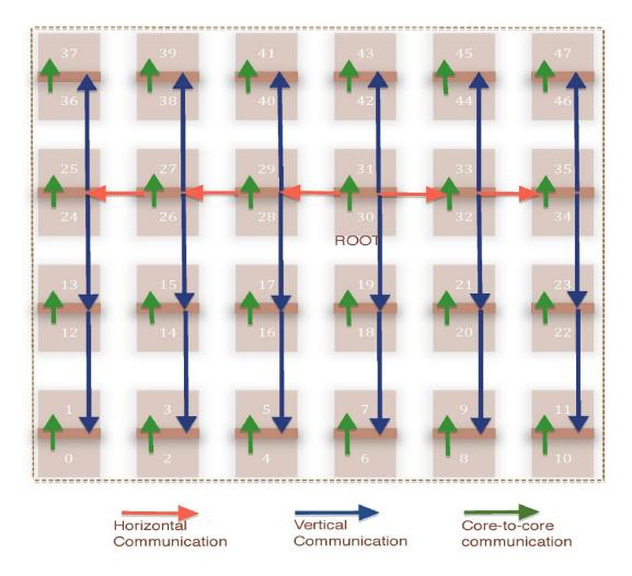
Figure 4.1: Communication pattern of Broadcast on Intel SCC
