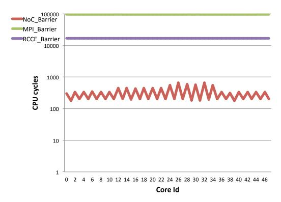
Figure 6.8: Comparison of *barrier()* for NoC\_Msg, RCCE and RCKMPI
