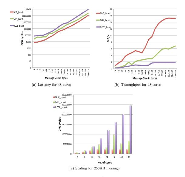
Figure 6.2: Performance analysis for *bcast()* of NoC\_Msg, RCKMPI and RCCE
