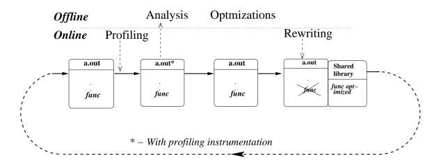
Figure 2.3: Cycle of Optimizations during execution lifetime
