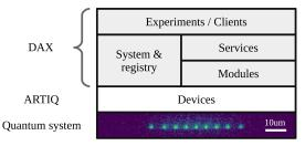
Fig. 1. Schematic overview of how DAX architecture combines with ARTIQ to control a quantum system, in this case a trapped ion device. This figure has been taken from [6].
