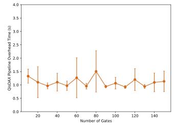
Fig. 9. QisDAX pipeline overhead. Each of these points indicates the average time taken by QisDAX to convert a Qiskit program into a DAX.program circuit, remotely submit it to CRYO-STAQ, and return the final result. Each data point on the plot was averaged over 10 samples, and the error bars indicate the standard deviation. The data shows a near-constant overhead of  $\sim 1.1$  seconds across increasing circuit depths.
