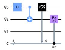
Fig. 2. A Qiskit circuit rendered using matplotlib renderer showing a Hadamard gate, a Controlled-X gate, a single qubit measurement to a classical register of size 3, and a Z rotation gate in order from left to right.
