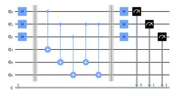
Fig. 6. Circuit for Simon's algorithm
