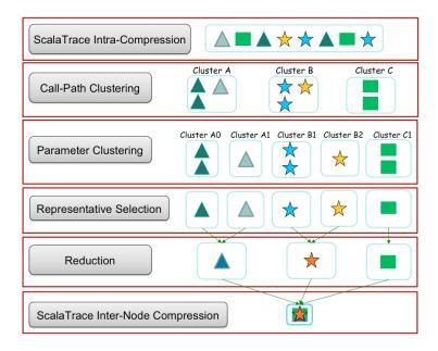
Figure 3: Overview of Proposed Clustering Algorithm
