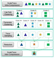
Figure 3: Overview of Proposed Clustering Algorithm
