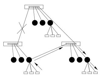
Network Flow in Presence of Line Fault
