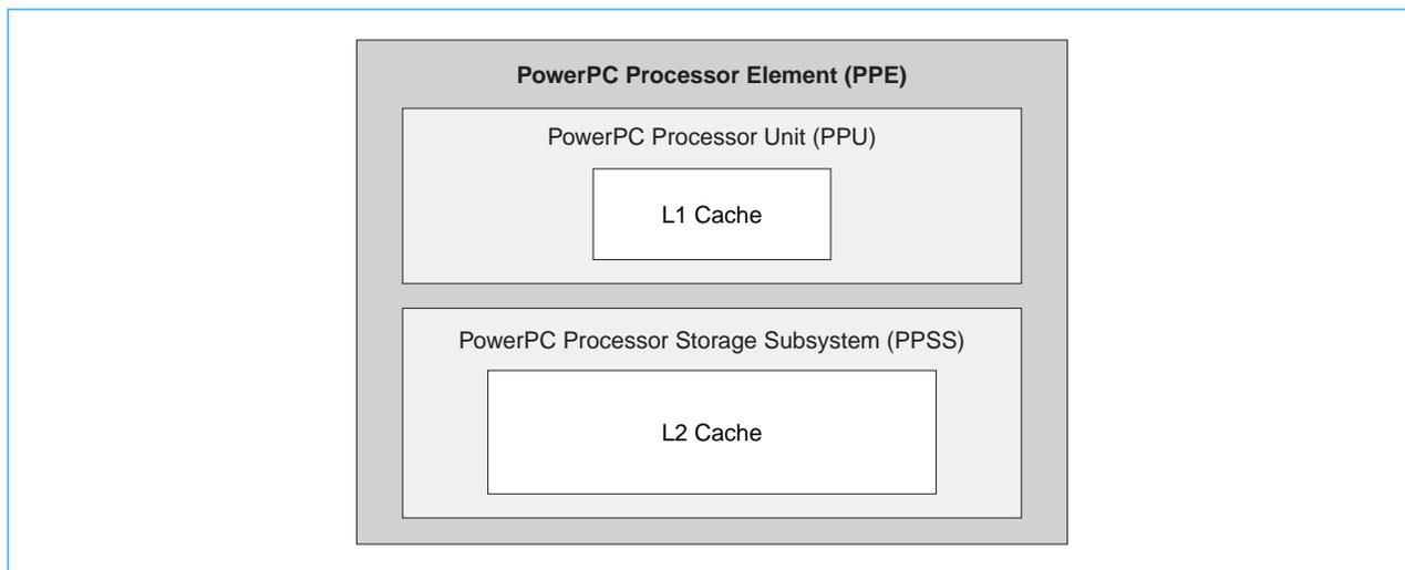
The PPU deals with instruction control and execution. It includes the full set of 64-bit PowerPC registers, 32 128-bit vector multimedia registers, a 32-KB level 1 (L1) instruction cache, a 32-KB level 1 (L1) data cache, an instruction-control unit, a load and store unit, a fixed-point integer unit, a floating-point unit, a vector unit, a branch unit, and a virtual-memory management unit.
