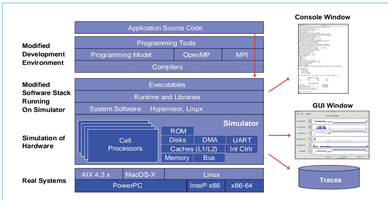
If accurate timing and cycle-level simulation are not required, the simulator can be used in its *functional-only mode*, running as a debugger to test the functions and features of a program. If cycle-level analysis is required, it can be used in *performance simulation* (or *timing simulation*) mode, to get accurate performance analyses. Simulator configurations are extensible and can be modified using Tool Command Language (Tcl) commands to produce the type and level of analysis required.
