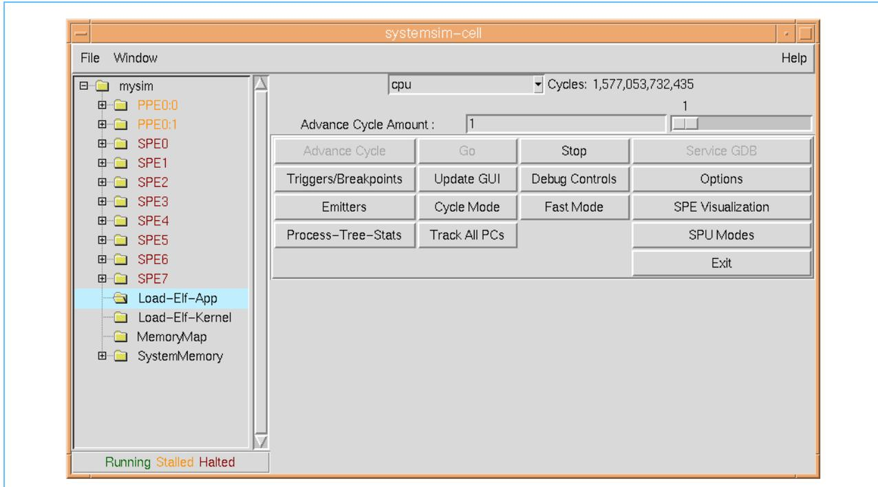
The main GUI window has two basic areas: the vertical panel on the left, and the rows of buttons on the right. The vertical panel represents the simulated system and its components. The rows of buttons are used to control the simulator.
