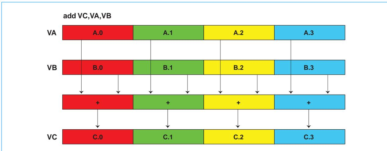
The process of preparing a program for use on a vector processor is called *vectorization* or *SIMDization*. It can be done manually by the programmer, or it can be done by a compiler that does *auto-vectorization*.
