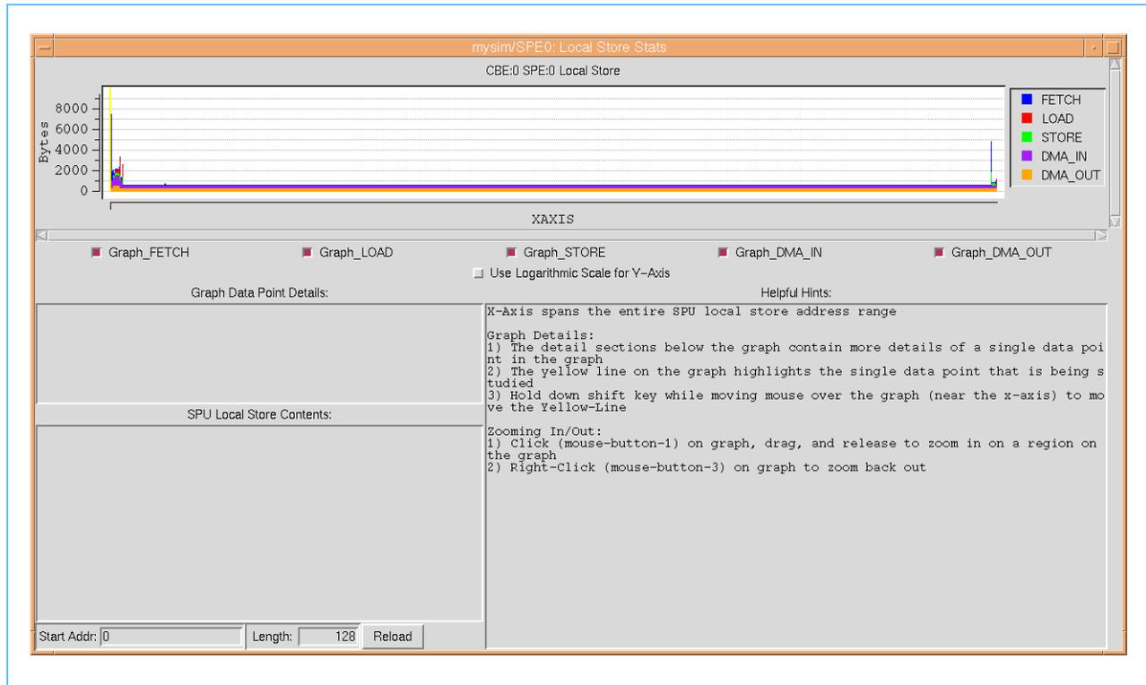
The last three items in an SPE folder represent actions to perform, with respect to the associated SPE. The first of these is *SPUStats*. When the system is stopped and you double-click on this item, the simulator displays program performance statistics in its own pop-up window.
