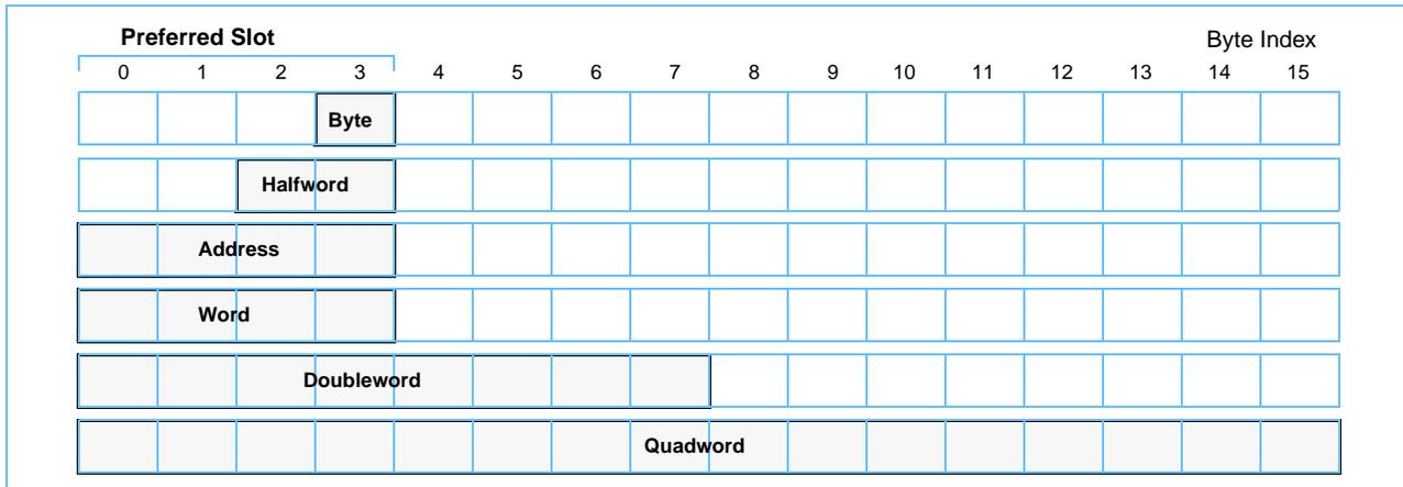
The SPE programming model defines the vector data types shown in *Table 3-5* for the C programming language. These data types are all 128 bits long and contain from 1 to 16 elements per vector.
