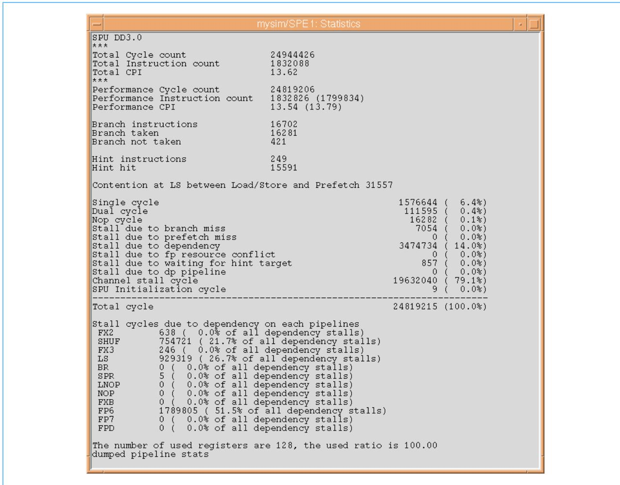
The next item in the SPE folder is labelled either *Model: instruction* or *Model: pipeline*. The label indicates whether the simulation is in *instruction mode*, for checking and debugging the functionality of a program, or *pipeline mode*, for collecting performance statistics on the program. The mode can be toggled by double-clicking the item. The SPU Modes button on the GUI can also be used as a more efficient way to set the modes of all of the SPEs simultaneously.
