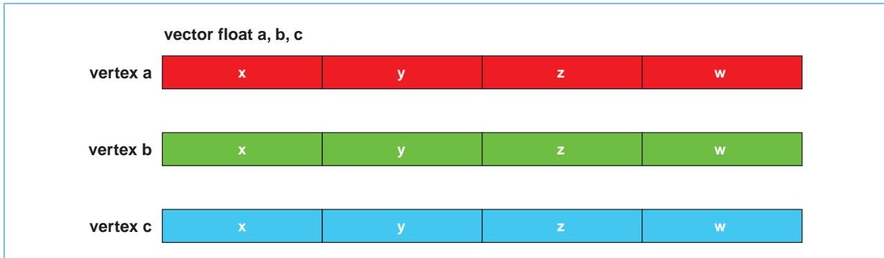
The data-packing approach shown in *Figure 3-5* often produces small code sizes, but it typically executes poorly and generally requires significant loop-unrolling to improve its efficiency. If the vertices contain fewer components than the SIMD vector can hold (for example, three components instead of four), SIMD efficiencies are compromised.
