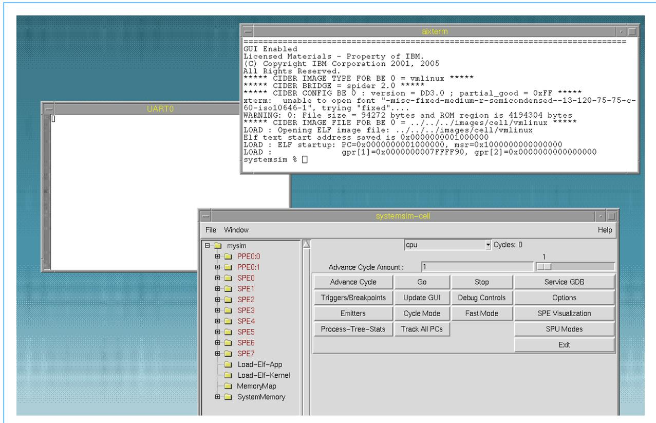
The window labeled *UART0* is a UART window that, when Linux boots effectively, becomes a Linux console window. The window in which the simulator was started (`./run_gui`) is the simulator command-line window. This is a command-line window (usually the serial port I/O) in the simulated Linux operating system on the simulated system. When the console window first appears, it is empty and there is no user prompt, because Linux has not yet been booted on the simulated system.
