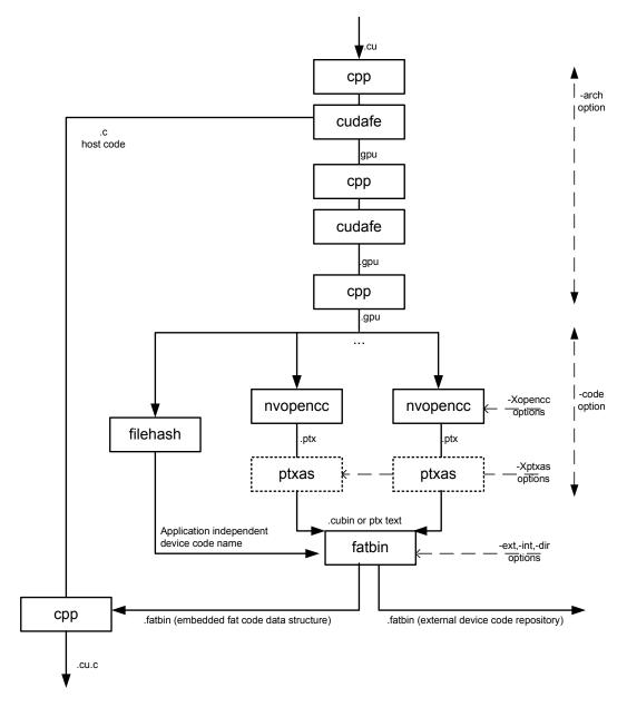
Figure 2: CUDA compilation from .cu to .cu.c
