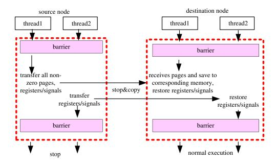
Figure 3.3: Process Migration without Precopy (Kernel Mode in Dotted Frame)
