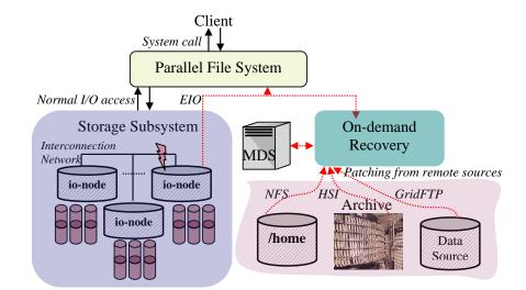
Figure 7.1: Architecture of on-the-fly recovery
