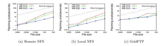
Figure 6.3: Patching costs for single OST failure from a stripe count 32. Filesize/32 is stored on each OST and that is the amount of data patched. Also shown is the cost of staging the entire file again, instead of just patching a single OST worth of data.
