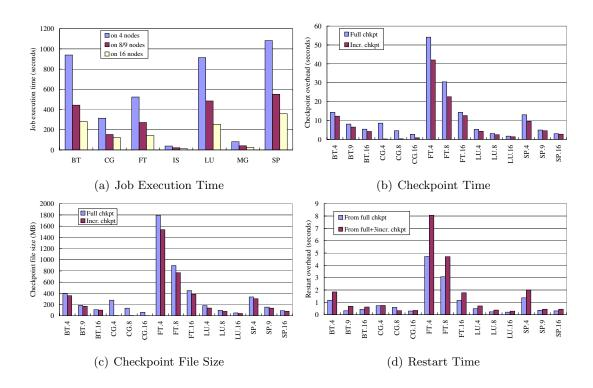
Figure 5.7: Evaluation with NPB Class C on 4, 8/9, and 16 Nodes
