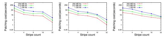
(a) Patching from remote NFS server (b) Patching from local NFS server (c) Patching from GridFTP server
