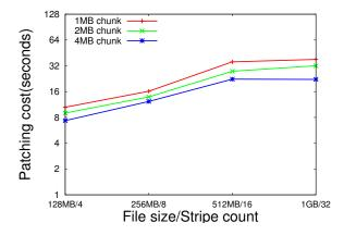
Figure 6.4: Patching from local NFS. Stripe count increases with file size. One OST fails and its data is patched.
