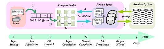
Figure 1.1: Event timeline of a typical MPI job's data life-cycle
