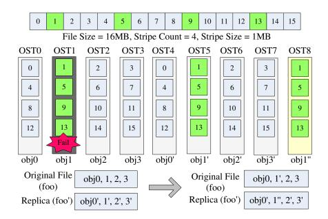
Figure 8.3: Objects of an original job input file and its replica. A failure occurred to OST1, which caused accesses to the affected object to be redirected to their replicas on OST5, with replica regeneration on OST8.
