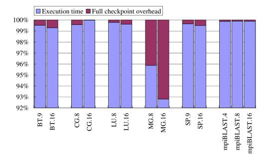
Figure 5.6: Full Checkpoint Overhead of NPB Class D and mpiBLAST
