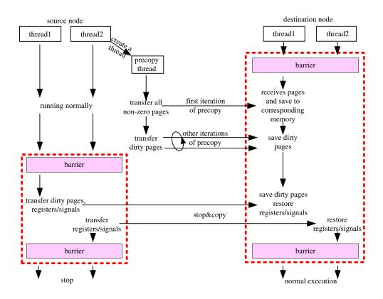
Figure 3.2: Process Migration with Precopy (Kernel Mode in Dotted Frame)
