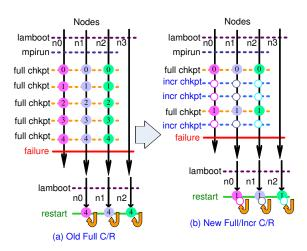
Figure 5.1: Hybrid Full/Incremental C/R Mechanism vs. Full C/R
