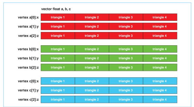
Figure 3-6. Structure-of-Arrays Data Organization for Four Triangles
