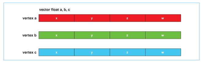
Figure 3-5. Array-of-Structures Data Organization for One Triangle
