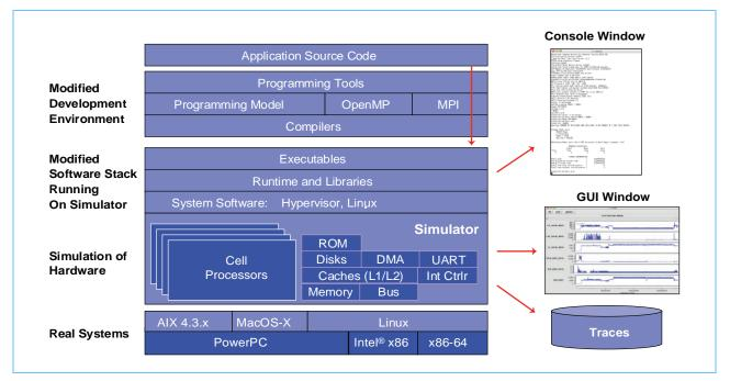
Figure 5-1. Simulation Stack
