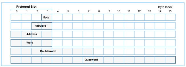
Figure 3-3. Register Layout of Data Types and Preferred Slot
