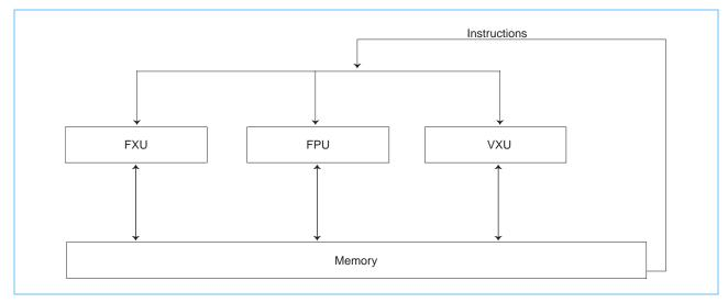
Figure 2-2. Concurrent Execution of Integer, Floating-Point, and Vector Units
