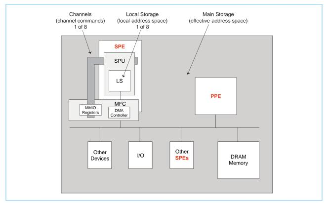
An SPE can only fetch instructions from its own LS, and loads and stores can only access the LS. An SPE or PPE performs data transfers between the SPE's LS and main storage primarily using DMA transfers controlled by the MFC DMA controller for that SPE. Software on the SPE's SPU interacts with the MFC through channels, which enqueue DMA commands and provide other facilities, such as mailboxes, signal notification, and access auxiliary resources.
