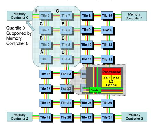
Figure 5.1: Memory Traffic Routing of a Quartile
