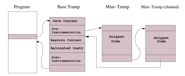
Figure 2.1: Inserting Instrumentation at a Point
