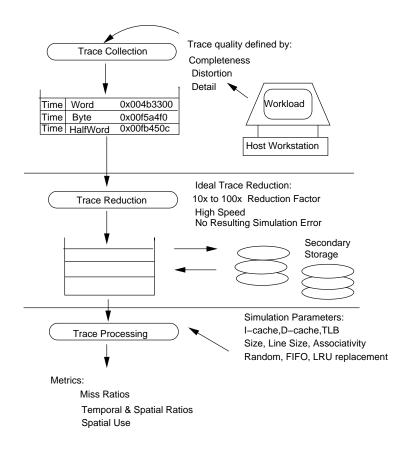
Figure 1.2: 3 Stages for Trace-based Simulators [29]
