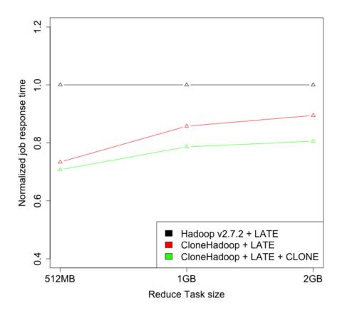
**Figure 7.6** Task size scaling:  $\beta = 1.2$ , *shape* = 2: Comparison of the normalized job response time for different reduce task sizes on a Terasort problem of size 128GB and reduce tasks of size 2GB.
