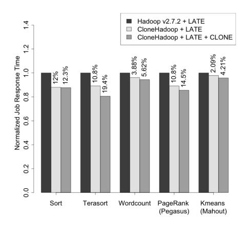
**Figure 7.8** Application Sensitivity:  $\beta = 1.2$ , *shape* = 2: Comparison of the normalized job response time for different application types.
