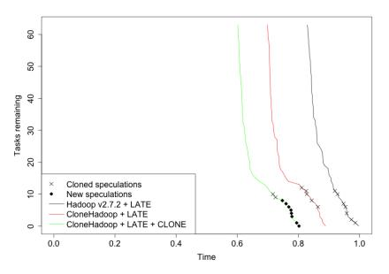
(**b**) Reduce Phase Completion: Reduce phase completion for the cloning-enabled speculator is staggered over a longer interval. However, since the reduce tasks start completing earlier, the overall effect on job response time is negligible
