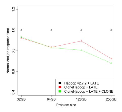
**Figure 7.7** Problem Scaling:  $\beta = 1.2$ , *s hap e* = 2: Comparison of the normalized job response time for Terasort jobs of different sizes, with map and reduce tasks configured to work on 4GB and 2GB of data, respectively. Cloned speculations improve performance with increase in problem size.
