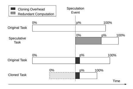
**Figure 1.1 Motivation for improving speculative execution:** Even when the speculative task is faster than the original task, it may have a later completion time due to the redundant work it has to complete. In contrast, cloning still leads to an overall faster completion time, even though cloning the task delays the original task
