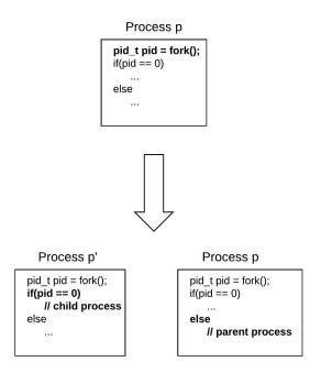
**Figure 4.2** fork() system call: The return value of fork() discriminates between the execution paths for the child and parent processes.
