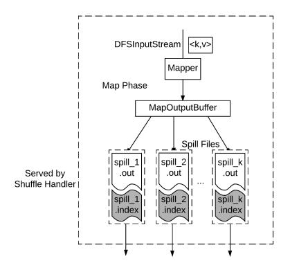
**Figure 5.2** Map Task workflow in CloneHadoop: instead of combining all map spill files at the end of the map task, each spill file is served by the Shuffle Handler.
