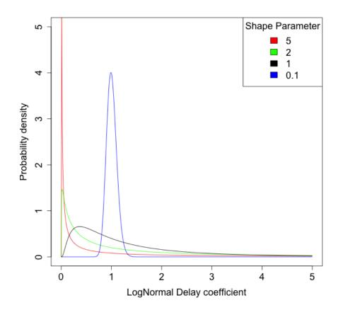
**Figure 7.1** Lognormal distribution and its variation with changes to shape: the varying tail characteristics allow us to test the sensitivity of our algorithm in different situations
