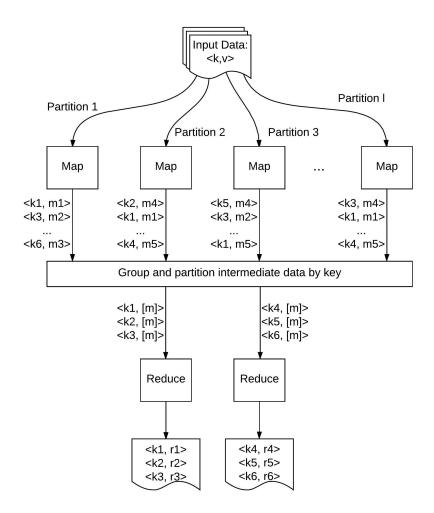
**Figure 2.1 Overview of MapReduce paradigm:** Each map subtask maps a partition of the input data set into intermediate key-value pairs. The intermediate data is grouped and partitioned by key to be handled by reduce phase. The lack of dependence between computations within a phase allows for high degrees of parallelism within a phase.
