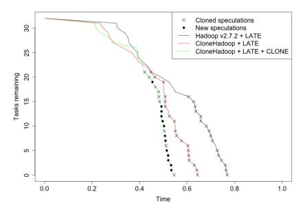
(a) Map Phase Completion: Map phase for the cloning-enabled speculator finishes earlier than LATE speculators
