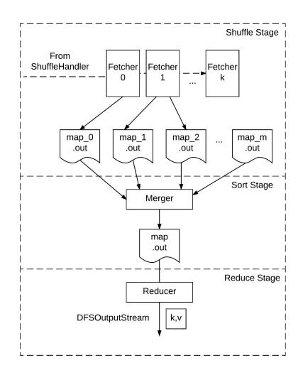
**Figure 2.3 Simplified Reduce Task workflow:** the Fetchers pull files from ShuffleHandlers on all nodes into memory. If the MapOutputFile does not fit into memory, it is spilled directly to disk. Depending on the size of the output files, the final merged file can contain a combination of disk and in-memory data.
