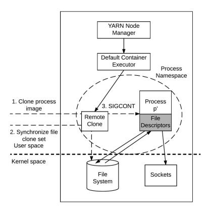
Figure 5.1 Integration of remote clone with Apache YARN Container Executor
