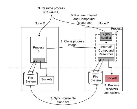
**Figure 4.3** Cloning design: Since the cloning algorithm works outside the context of the cloned process, we use a signal handler to modify the cloned process' state.
