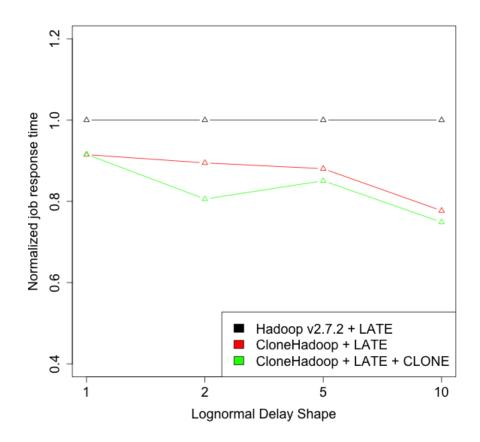
**Figure 7.4** Straggler Distribution analysis:  $\beta = 1.2$ : Comparison of the normalized job response time for varying straggler distribution shapes on a Terasort problem of size 128GB.
