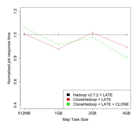
**Figure 7.5** Task size scaling:  $\beta = 1.2$ , *shape* = 2: Comparison of the normalized job response time for different map task sizes on a Terasort problem of size 128GB and map tasks of size 4GB.
