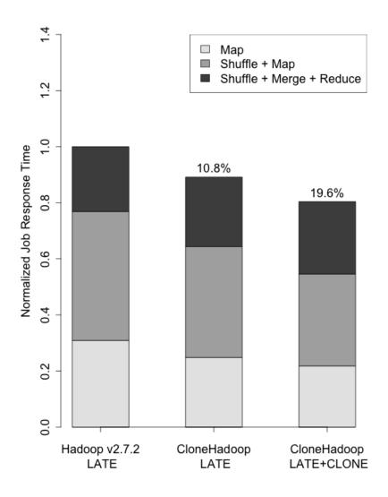
**Figure 7.2** Job Runtime Analysis:  $\beta = 1.2$ , *shape* = 2: Comparison of the normalized job runtime for a Terasort problem (128GB, 32 map tasks, 64 reduce tasks). We observed a standard deviation of not more than 1% in job response times. Since the task runtime distribution is short-tailed, cloning speculations improve the overall job run-time: nearly 11% for CloneHadoop and 20% for the cloning speculator.
