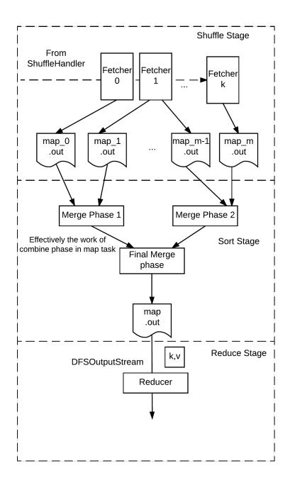
**Figure 5.3** Reduce Task workflow in CloneHadoop: since the reduce task now fetches spill files instead of map output files, the reduce task may have to undergo several phase of running the combiner.
