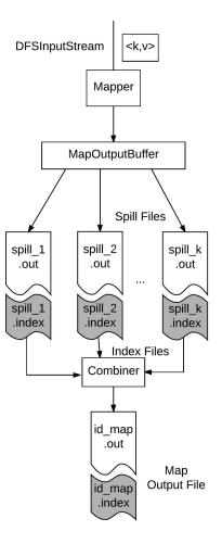
**Figure 2.2 Simplified Map Task workflow:** the MapOutputBuffer spills key-value pairs to disk when it runs out of memory. Once all key-value pairs have been processed, the buffer spills the remaining data to disk and the combiner collects all spill files into a single map output file.
