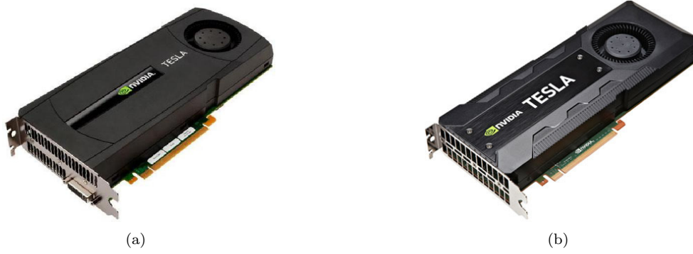
Figure 1: The Nvidia Tesla GPGPUs used in the present work: (a) C2050 (448 stream processors, 3GB memory); (b) K20c (2496 stream processors, 5GB memory).
