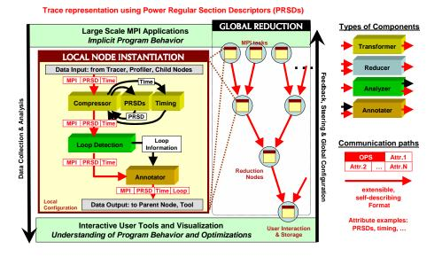
Figure 1: Interaction of Components
